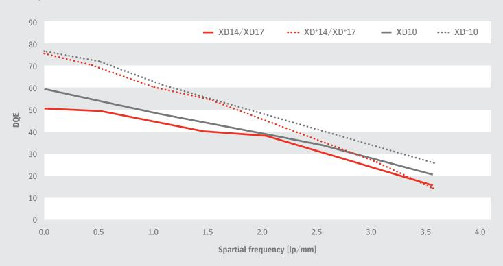
Detective quantum efficiency (DQE) of the Dura-line detectors, measured according to IEC 62220-1 (standard beam quality at 2.5μGy). Improved IQ at low dose for the XD+ line: DQE 75% @ 0 lp/mm\*.
