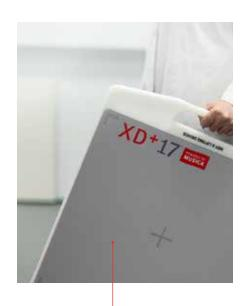
Click-On ergonomic handle can be mounted on the detector, for even easier transport and handling.
