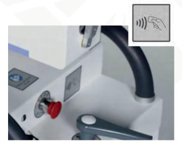
Zero dose centering thanks to laser localizers on X-ray tube and on flat panel detector side.
