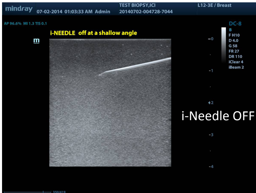
Biopsy needle with i-Needle turned off demonstrated at a shallow angle
